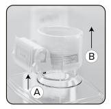
(A) Grab refill collar from below battery. (B) Pull straight upward to remove. Dispose/recycle PET bottle.
